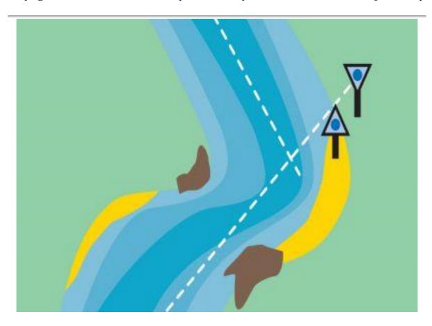
The lead marks are two separate navigation aids (one in the foreground and one placed further back on the shore) which, when aligned, provide the correct course for the vessel to steer.
